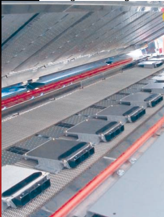
2 ways conveyor with combined loading / unloading zones
