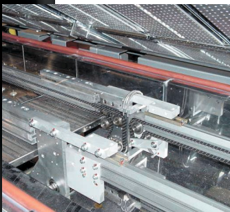
Buffer conveyor for fast extraction of the product to the test zone.
